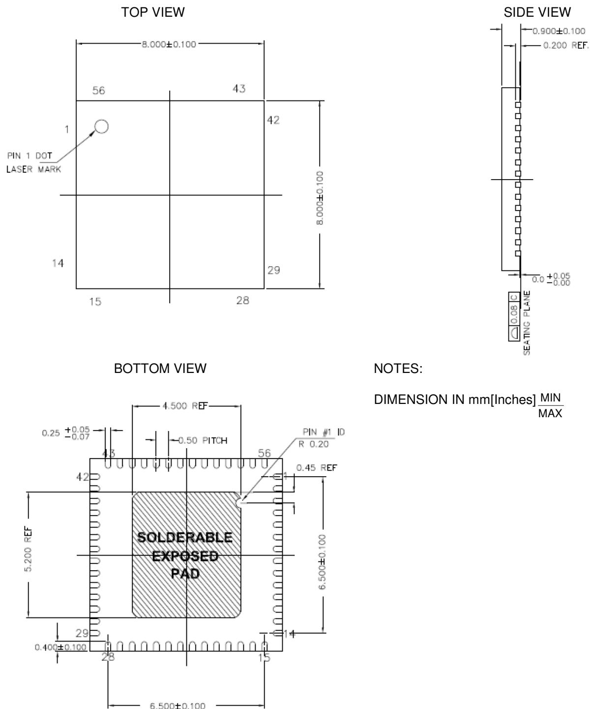
SK5102-LT 56-Lead (8x8mm 1.0 MAX) Saw QFN
