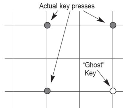
When an external hardware (normally adding diode to each key switch) is used, the ghost key mechanism can be disabled via FlexMatrix Editor. This feature enables N-key rollover designs.
